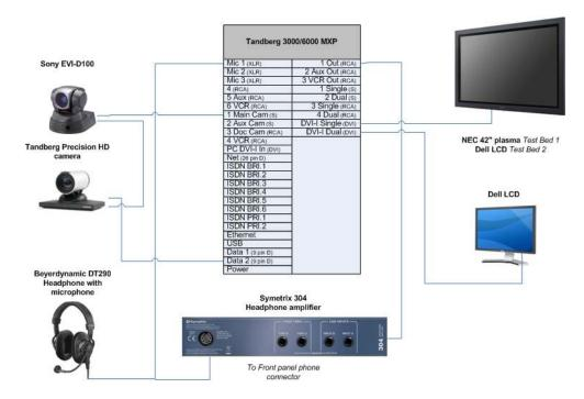
Figure 6. Codec Test Rack Setup
